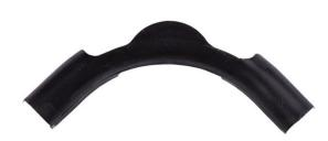
The turn lock is used when laying a pipe for a warm floor to avoid fractures when making a 90° turn. It is used for pipes with a diameter of 16 mm and 20 mm.
